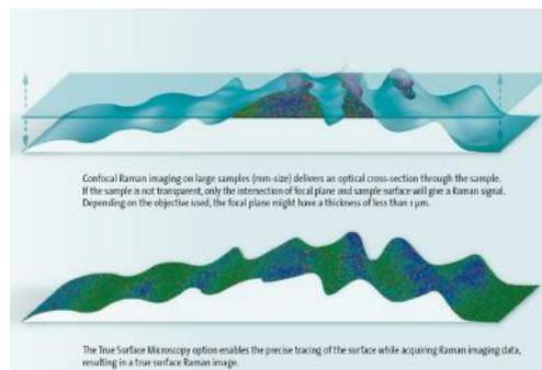
Above (without TrueSurface®): When imaging rough surfaces in confocal imaging mode only parts of the sample are in focus. Below (with TrueSurface®): Following the topography in confocal imaging mode enables the surface to always stay in focus.
