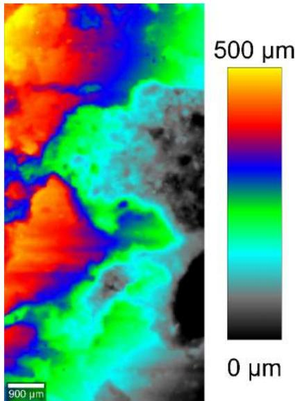
Fig. 3: Topography of the sample as recorded using the TrueSurface® extension of the alpha500 R.
