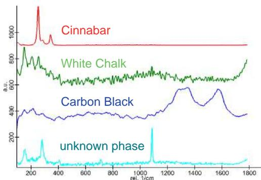
Fig. 5: Spectral components Raman analysis. The spectra could be identified as: Red = Cinnabar; Green = White Chalk (CaCO<sub>3</sub>, Calcite); Blue = Carbon Black; Turquoise = unknown phase.
