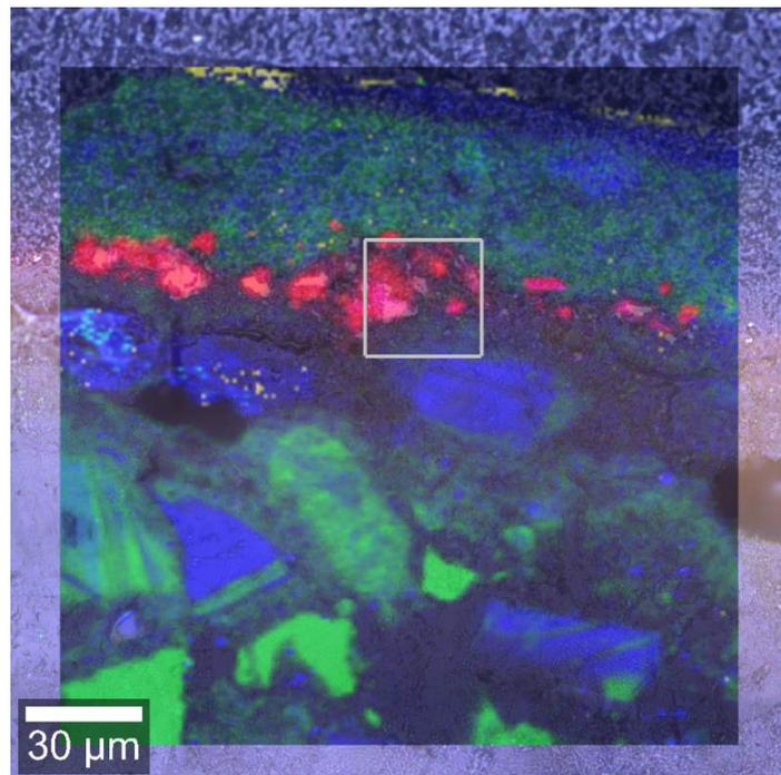
Fig. 10: Color-coded confocal Raman image overlaid on a white light image of a cross section of the sample. The colors correspond to the colors of the spectra in Fig. 11. The frame indicates the area at which a consecutively second scan was performed.
