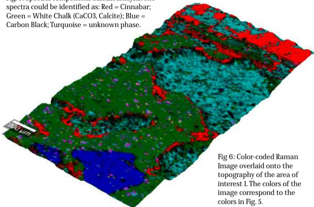
Fig 6: Color-coded Raman Image overlaid onto the topography of the area of interest 1. The colors of the image correspond to the colors in Fig. 5.
