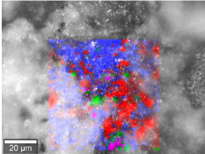
Fig. 8: Color-coded Raman image overlaid on the white light image of the area. Color coding: Ochre crystals - Red; Calcium carbonate binder mixed with ochre - Blue; High level of fluorescence - Green.
